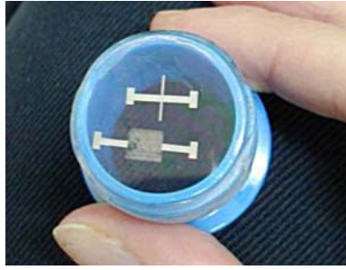
Fig. 3.23: Realization of two gold bottom contact OFETs on Mylar. Image taken from [60].
