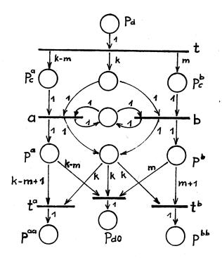
${\bf k}$ ,  ${\bf m}$  ( ${\bf k}$ > ${\bf m}$ ) are to be specified depending on the control. The place  ${\bf p}_{d0}$  will be marked iff transition a fires exactly k-m times and d fires exactly m times (the sum of their firings during one test run is always k). This has to be the case if  ${\bf p}_c^a$  and  ${\bf p}_c^b$  were clean (i. e., the contents of c were zero) before starting the test run by firing t.
