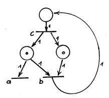
We use the partition  $\{\{a,c\}, \{b\}\}\}$  and suppose that decisions are made for a by  $A_1$  and for b by  $A_2$ . After the firing of b, transition a is not firable any more, but transition c becomes firable. Nevertheless, c is not allowed to fire under the control because we still have  $V_1 = \{a\} \neq \emptyset$  and thus  $A_1$  is not in the position for a new computation in favour of c. Such effects are reflected by the following definitions.
