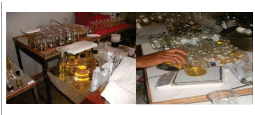
Figure 4.20: The oil expressed from the conditioned seed is settled, decanted and weighed to determine the efficiency of expression.
