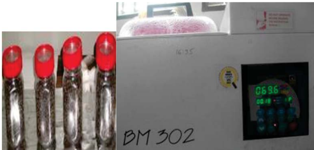
Figure 5.29: Kilning jar filled with nigerseed, for conditioning in temperature-time programmable water bath (with precision of 0.05°C).
