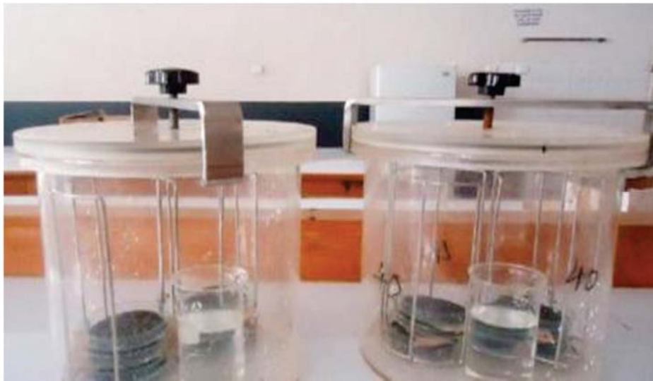
Figure 4.15. The equilibrium relative humidity chamber with screw clump rubber seal (the salt solutions in beaker and the two varieties of nigerseed in triplicate inside the chamber).
