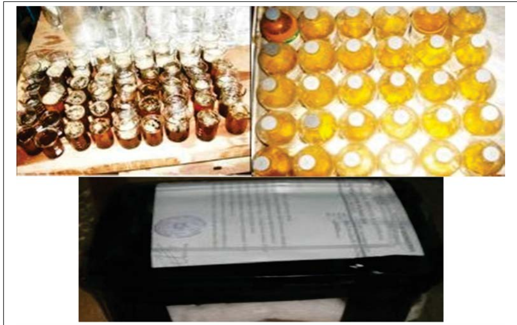
Figure 4.13: Oil expressed, settled and decanted to vials from the respective experimental field plot and packed (ready for laboratory examination).
