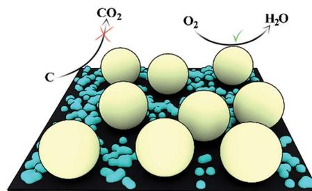
Fig. 5 Schematic representation of the SnO<sub>2</sub>(blue)/Pt(yellow)/CFs (black) surface.
