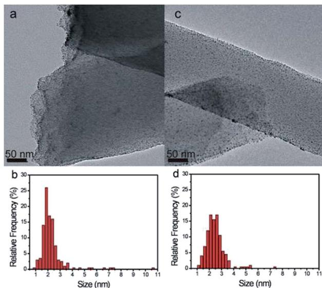
Fig. 1 (a and c) TEM images and (b and d) particle distribution obtained from TEM analysis of (a and b) Pt/CFs, (c and d) SnO<sub>2</sub>/Pt/CFs before cyclic voltammetry.
