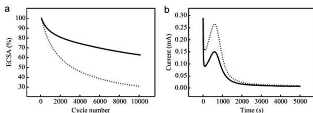
Fig. 6 (a) ECSA of Pt/CFs (dotted line) and  $\text{SnO}_2/\text{Pt}/\text{CFs}$  (full line) calculated from cyclic voltammetry at  $50 \text{ mV s}^{-1}$  in a  $\text{N}_2$  saturated  $0.5 \text{ M H}_2\text{SO}_4$  solution every 100 cycles performed at  $100 \text{ mV s}^{-1}$ . (b) Oxidation/corrosion characteristics for Pt/CFs (dotted line) and  $\text{SnO}_2/\text{Pt}/\text{CFs}$  (full line) at  $1.4 \text{ V/RHE}$ .
