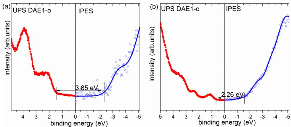
Figure S6. UPS / IPES spectra of 10 nm (a) DAE1-o, (b) DAE1-c films on ITO substrates, from which the charge transport gaps (3.85 eV for DAE1-o, 2.26 eV for DAE1-c) of the DAE1 layers were determined. For the IPES measurement, the sample and filament current were kept at an extremely low level ( $I_{\text{sam}} < 0.1 \mu\text{A}$ ,  $I_{\text{filament}} = 1.03 \text{ A}$ ) to minimize sample damage.
