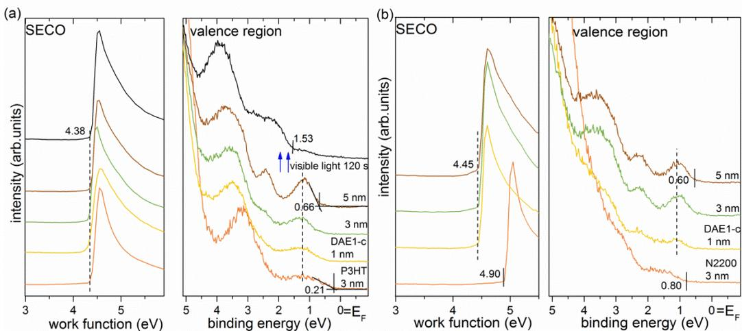
Figure S4. (a) UPS spectra of DAE1-c films with incremental deposition thickness on P3HT substrates. After 5 nm thick deposition, samples were irradiated by visible light ( $\lambda > 450$  nm); during this process, molecules switched from closed to open form. (b) UPS spectra of DAE1-c films with incremental deposition thickness on N2200 substrates.
