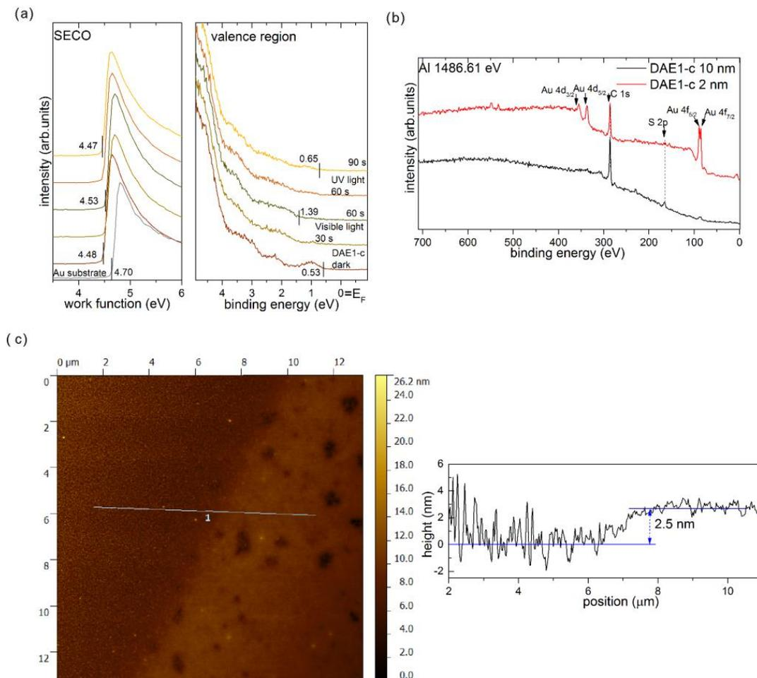
Figure S2. (a) UPS spectra of 2 nm DAE1-c film, switching process was achieved by the irradiation of visible and ultraviolet light, respectively. (b) XPS survey spectra of thick and ultra-thin DAE1-c film deposited on Au substrate. The signals of gold (e.g., Au 4f) indicate film thickness differences. (c) Topography image of ultra-thin DAE1-c layers on Au surface as measured by AFM. Film thickness was measured by partially wiping away surface molecules using ethanol.
