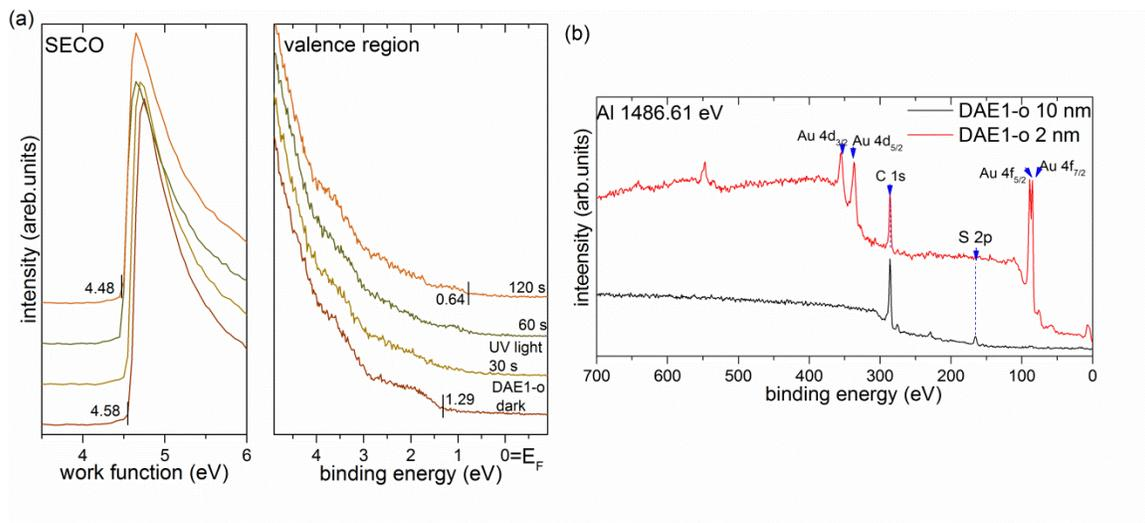
Figure S3. (a) UPS spectra of 2 nm DAE1-o film, switching process was achieved by the irradiation of UV light. (b) XPS survey spectra of thick and ultra-thin DAE1-o film deposited on Au substrates.
