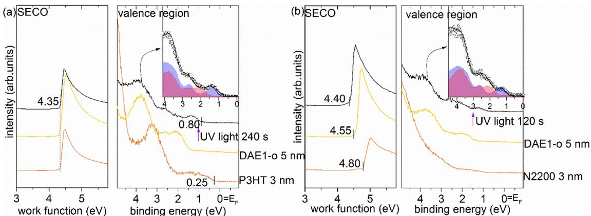
Figure S5. UPS spectra (valence and SECO regions) of 5 nm thick DAE1-o films on (a) P3HT and (b) N2200, and light switching induced changes. Inset: deconvolution of sample spectrum (open circles) after UV light irradiation with DAE1-c and DAE1-o contributions (sum given by the black line, which is composed by 45% of DAE1-o and
