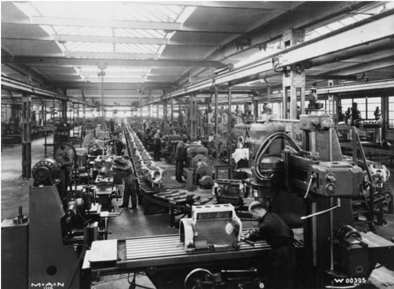
Fig. 4. Inscription on back: Factory machinery MAN 1938, neg. no. 1429-9-13, photo W 00395, industrial workstations for truck engine construction, Building E 1 A, crankcase assembly. Source: Historisches Archiv der MAN, Augsburg.
