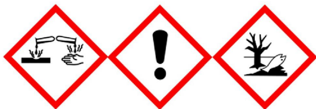
FIGURE 4 GHS-Gefahrstoffkennzeichnung of zinc chloride. GHS-Gefahrstoffkennzeichnungen are used in Germany to label hazardous chemicals. Different labels identify different properties. The properties shown here are corrosive (left), harmful (middle) and harmful to the environment (right).
